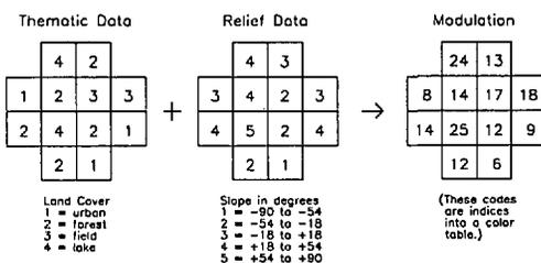
Figure 1. Generating modulated map codes.
